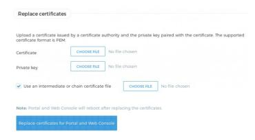
The Web Console interface removes the need for complex manual procedures through the command-line interface for replacing digital certificates in Nexthink Appliances, at least for the most common cases.
