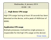
The tooltip displays the peak of CPU usage on the device during a time interval when the CPU usage is above 80%. Then it compares the peak value to the total capacity of the CPU. A 100% usage corresponds to the capacity of a single core CPU. You can get more than 100% usage in CPUs with multi-core or hyper-threading technologies:
