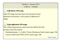
The lower part of the tooltip displays a list of processes that consumed more than 50% of the CPU processing power (40% for the system process) for at least 30 seconds during the selected time interval. Processes are ordered in the list by their contribution to the CPU load from the most to the least demanding. The higher part shows the total CPU usage on the device during the same time interval.
